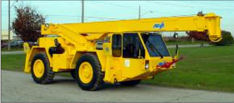
"The AT3035M Series- 7½ Ton Rough Terrain Crane preferred by the USAF"
