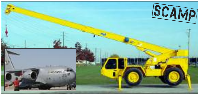
"OPTIONAL: Available 94 inch axle making it the ideal crane for transportation with Chinook on C-17"
