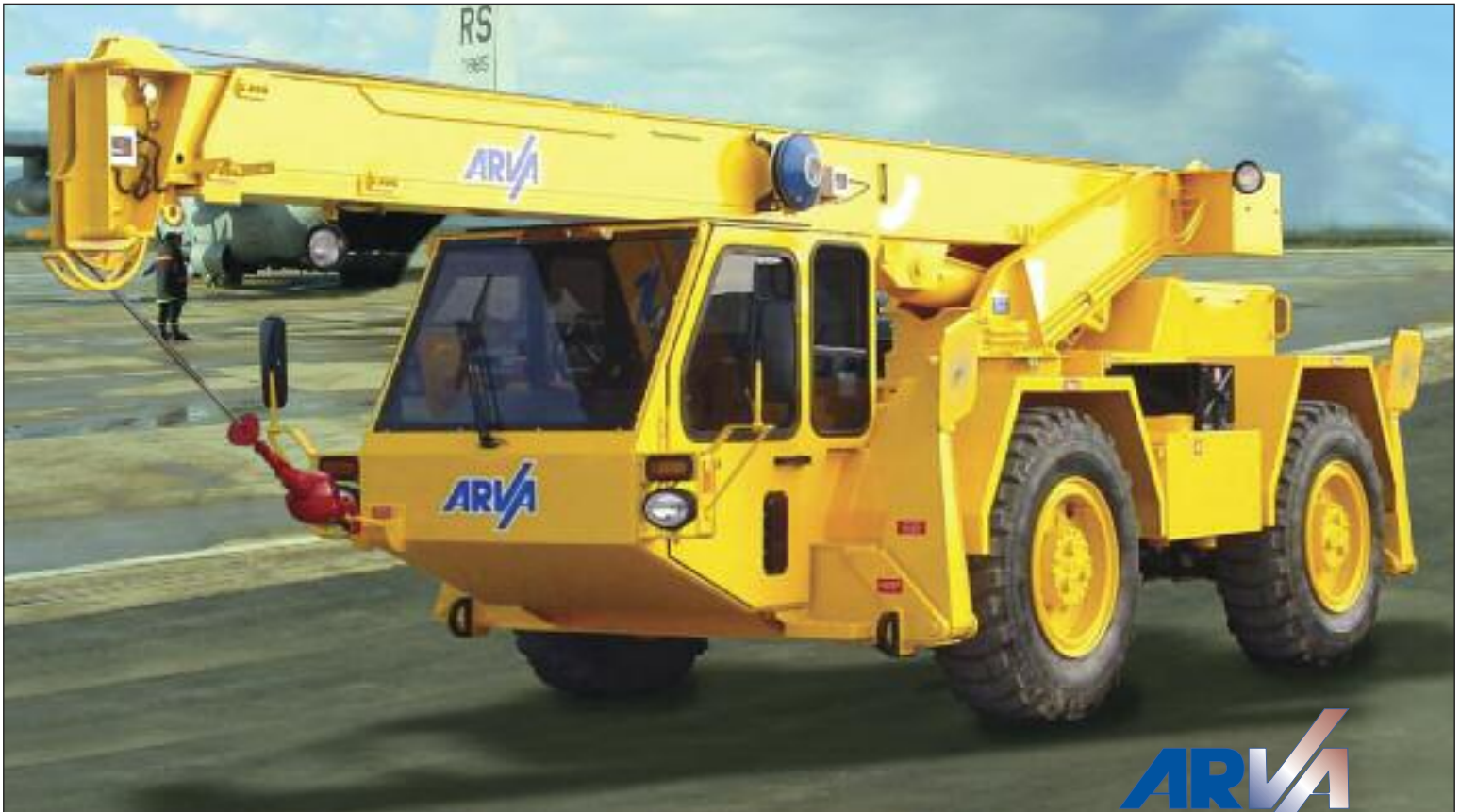
"OPTIONAL: Available 94 inch axle making it the ideal crane for transportation with Chinook on C-17"
